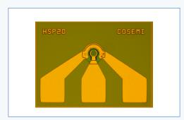
Cosemi's LPD3030 is a mesa-structured, InGaAs/InP-based PIN photodiode offering high responsivity, low dark current and low capacitance for high bandwidth, high performance optical receiver designs.
